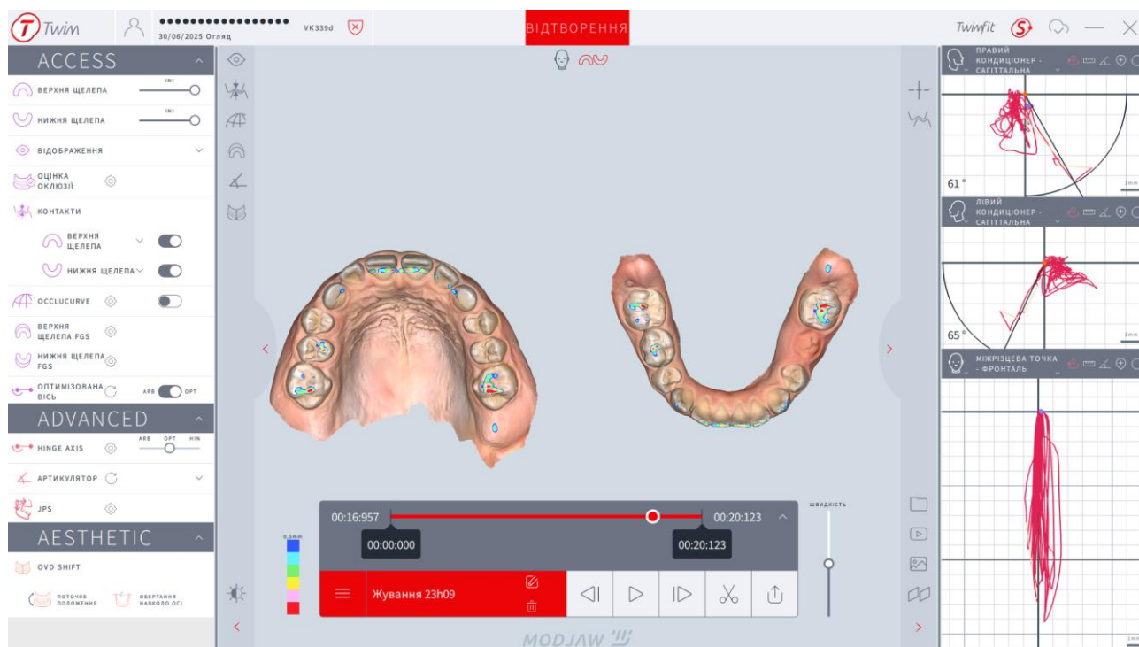
Figure 2. Representative visualization of masticatory function recorded with the Modjaw digital system. The image demonstrates synchronized three-dimensional maxillary and mandibular models with occlusal contact mapping, incisal point trajectory, and bilateral sagittal condylar movement curves during a chewing cycle
